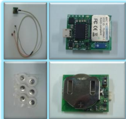
Figure 3. Sensor developed to capture both inclination of some part of the child body and the muscular effort (sEMG signal).
