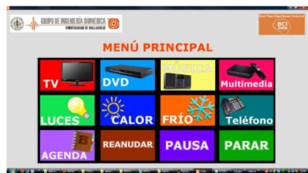
Figure 1. Main Menu of the domotic BCI application. The user can choose between different devices usually present at home: TV, DVD, telephone, heater, lights, etc.
